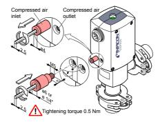
Insert the tube into the instant push-in fitting until the mechanical stop is reached. Check that it is correctly mounted by slightly pulling.
